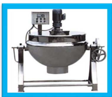
Figure 12: Jam Kettle (an example for small scale manufacturing)
