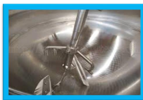
Figure 12: Jam Kettle (an example for small scale manufacturing)
